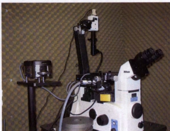
Figure 3.4: Image of Asylum Molecular Force Probe 3D AFM.
